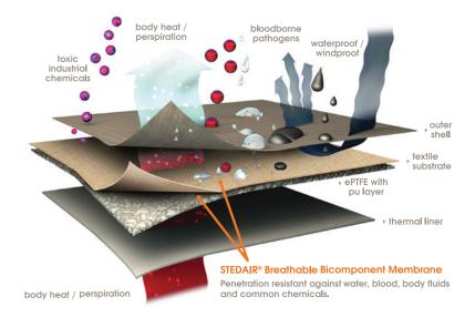
The overall technology allows for extensive moisture vapor transmission because the vapor molecules are small enough to freely diffuse through the voids of the membrane while the water molecules are too big to penetrate through the membrane. In addition to the excellent physical properties of the barrier, Stedair® Moisture Barriers provide protection against toxic industrial chemicals and hydrocarbon oxidizing agents. These very small but harmful chemicals are prevented from penetrating through
