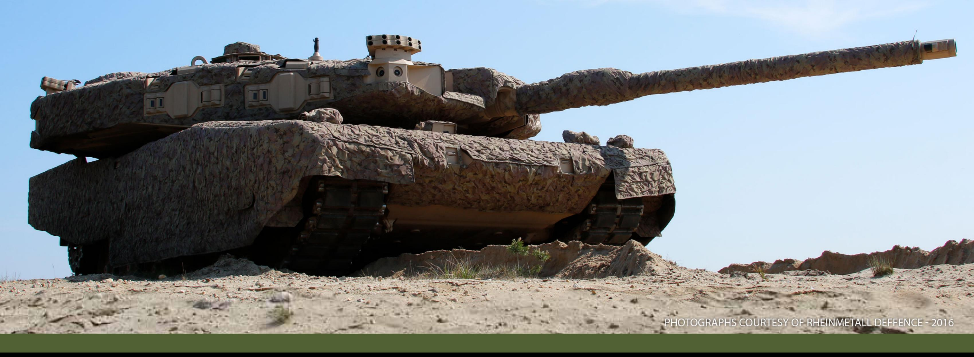
**SOLAR SHIELD**<sup>®</sup> is a 3D multi-laminated spacer fabric which provides significant solar heat and load reduction. The layered construction allows multispectral signature management against infrared, visual, and UV detection.
